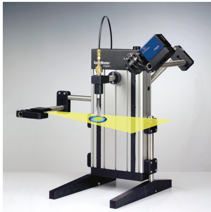
light sheet inspex configuration
