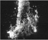
up to 4000 full frames **EngineMaster High-Speed** imaging system incorporates a state-of-theart CMOS camera synchronized to a diode pumped solid state laser. The system can record image sequences with up to 12 kHz frame rate (corresponds to 2000 rpm with 1° resolution). Each frame can be synchronized to crank angle or time based upon an external start trigger. A recording contains up to 4000 frames with 1024 x 1024 pixels each.
